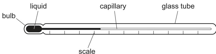
Which single change to the design of the thermometer increases the sensitivity?
